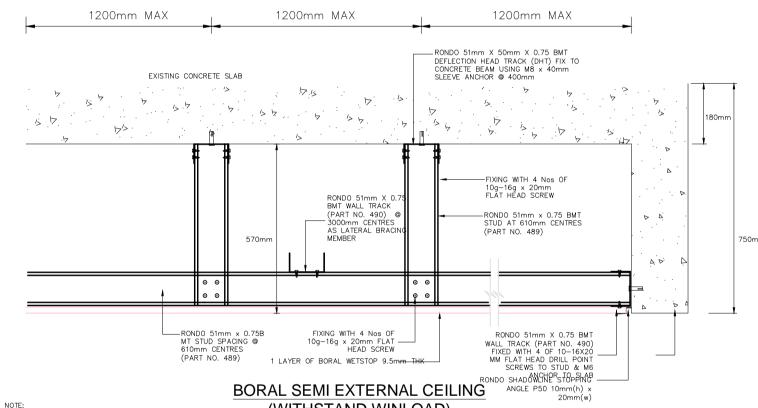
(WITHSTAND WINLOAD) WEIGHT OF CEILING SYSTEM = APPROX. 7.7KG/M2 EXTERNAL PRESSURE:
